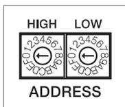
The address selection switch allows setting the amplifier's network address, which, within a CAN-network, can range from 01 to 250 (FA hex). Caution: Each address may exist only once within a network. Otherwise network conflicts might occur. Address setting has to be performed in hexadecimal code. The selection switch LOW represents the low-value digit while the HIGH-switch represents the high-value digit.
